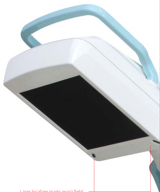
Laser localizer marks exact field of fluoroscopy to decrease in order exposure.
